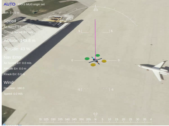
Figure 5. MAVCesium visualization of ArduCopter FITL. The interface displays the simulated vehicle attitude, position, and flight status using telemetry.
