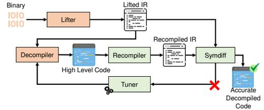
Figure 1: D-HELIX pipeline: D-HELIX extracts symbolic models for *Lifted IR* and *Recompiled IR*, and compares the symbolic models using a constraint solver. For semantically inequivalent models, D-HELIX uses the TUNER to fix the decompiled code.
